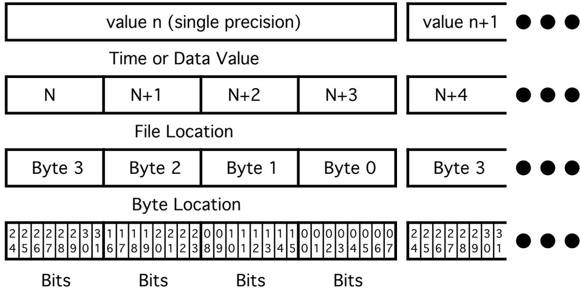
Figure 3.3.1-1 Floating Point File Storage Layout
